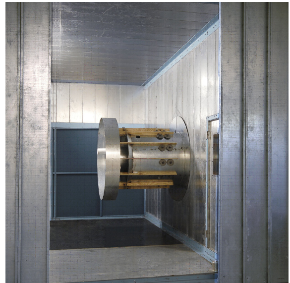
Test Duct Wind box with Burner Mock-up
